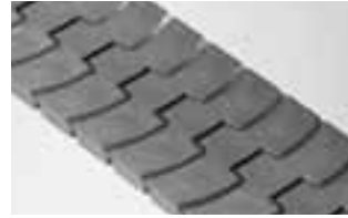
SERIES 4009 FLAT TOP • Hinge driven • Closed hinge • Sideflexing • 1.00 in. (25.4 mm) pitch • Available width: 83.8 mm (for parallel running at 85 mm)
