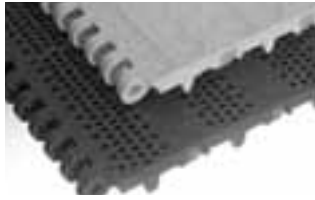
SERIES 800 • Center-driven • Open hinge • 2.00 in. (50.8 mm) pitch
