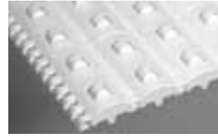
SERIES 800 ROLLER TOP • Center-driven • Open hinge • 2.00 in. (50.8 mm) pitch
