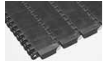
SERIES 900 • Center-driven • Closed hinge • 1.07 in. (27.2 mm) pitch
