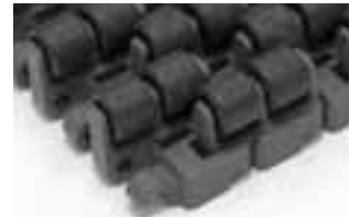
SERIES 1700 TRANSVERSE ROLLER TOP • Center/Hinge-driven • Closed hinge • 1.50 in. (38.1 mm) pitch
