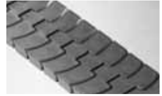
SERIES 4014 FLAT TOP • Hinge driven • Closed hinge • Sideflexing • 1.00 in. (25.4 mm) pitch • Available width: 83.8 mm (for parallel running at 85 mm)
