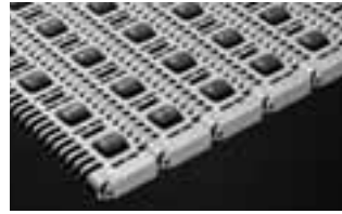
SERIES 400 0.85" TRANSVERSE ROLLER TOP • Center-driven • Closed hinge • 2.00 in. (50.8 mm) pitch
