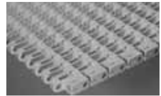
SERIES 1700 NUB TOP • Center/Hinge-driven • Closed hinge • 1.50 in. (38.1 mm) pitch
